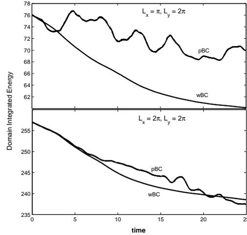
**Fig. 1.** The total energy (in arbitrary units) in the SB as a function of time (in units of  $\Omega_0^{-1}$ ). In the upper panel the size of the SB is  $L_x = \pi$  and  $L_y = 2\pi$  and the result of the calculation with PBC is compared with the one using WBC. In the lower panel the same is shown for a SB having a double shear-wise extent. In both cases the simulations are started with the same initial conditions
